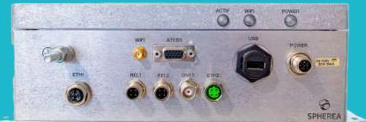
In 2015 a serious TGV accident occurred near Eckwersheim, in the Grand Est region. This led to the creation of the ESVE system, designed to autonomously monitor the train's speed in relation to its position on the track during testing. In the event of overspeed, it automatically triggers the emergency braking system to ensure safety.
