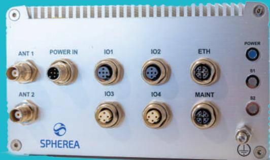
A new generation of on-board real-time monitoring system ensuring the continuous and secure activation of the TVM railway signaling system.
