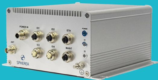
SFINX is a real-time embedded computer with a wide range of supported I/Os and peripherals running a SPHEREA's U-TEST® real-time core.
