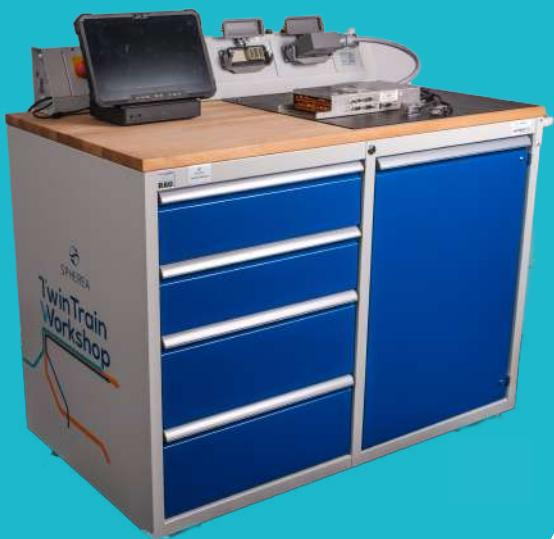
SPHEREA's TwinTrain Workshop is a standardized solution for testing a wide range of electrical and electronic components in rail vehicles. Despite their varied functions, many components share similar interfaces. The system uses generic measurement and stimulation electronics, requiring only an adaptation cable to test different Devices Under Test (DUTs). This enables fast, flexible deployment of new applications.
